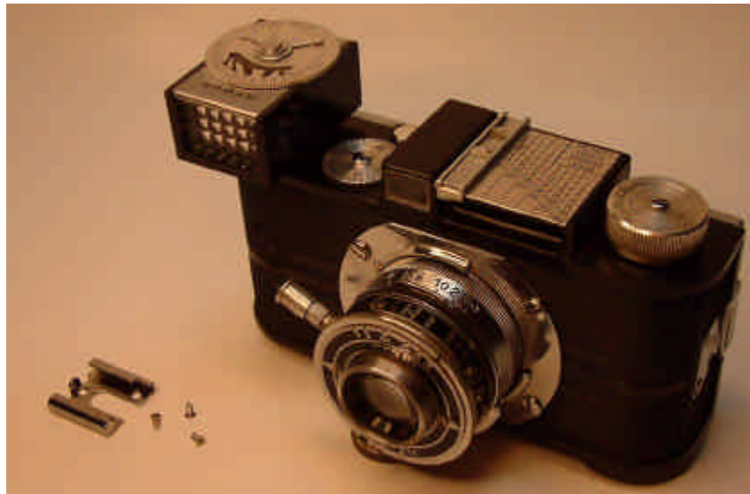
Fig 8-2: An Argus LS-3 light meter mounted by cold shoe on an Argus A2F
